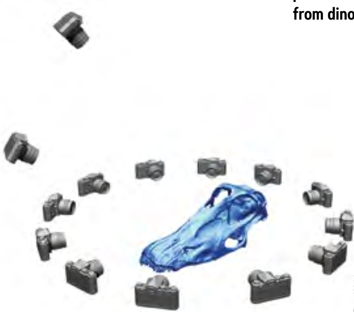
Schematic of the process of digitising a Diplodocus skull using digital photogrammetry, in which a large number of slightly overlapping photographs that cover the entire surface of the fossil are taken. These images are then processed in a computer to obtain a large number of homologous points between all the photographs, which are used to generate a virtual surface.
