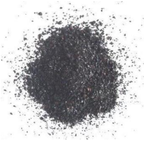
Figure 2. Blast furnace dust (BFD)
