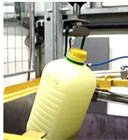
Figure 3. Drop test method for handles resistance.
