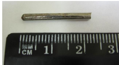
Figure 1. BMG rod obtained by copper mold casting.
