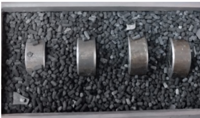
Fig. 2. Hermetic box for carburizing
