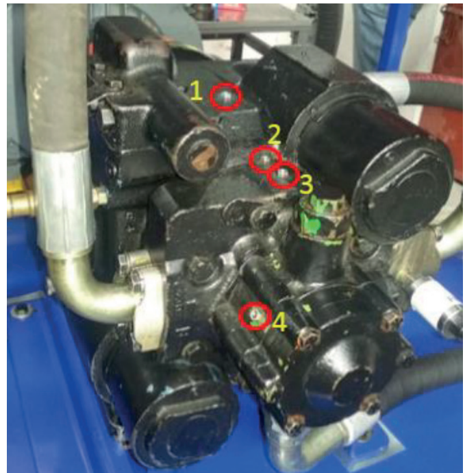
Fig. 3. Positions taken for vibration measurement.
