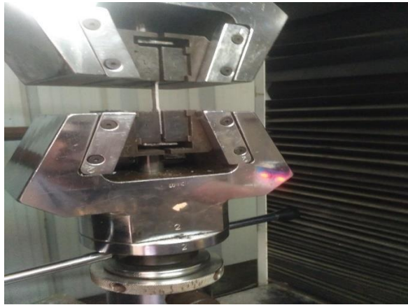
Figure 9(b) Material holding under 2 jaws
