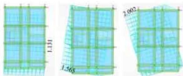
Figure 12. Maximum displacements for soil A (cm): 1 st mode on the left, 2 nd mode in the middle, and 3 rd mode on the right.
