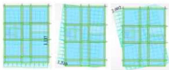
Figure 14. Maximum displacements for soil E (cm): 1 st mode on the left, the 2 nd mode in the middle, and the 3 rd mode on the right.
