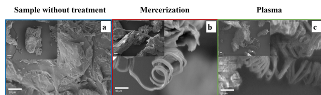
Figure 5. Morphological analysis: a) Image of the sample without treatment; b) Chestnut husk fibers with mercerization treatment in NaOH; c) Chestnut fibers with 80 mA plasma treatment.
