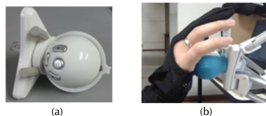
Figure 4. a) Grip adaptation of the kinesthetic interface, b) coupling between HaptTech and the Novint Falcon interface Source: Authors
