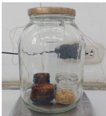
Figure 1. Respirometry setup for biodegradation and stability of bioadsorbents
