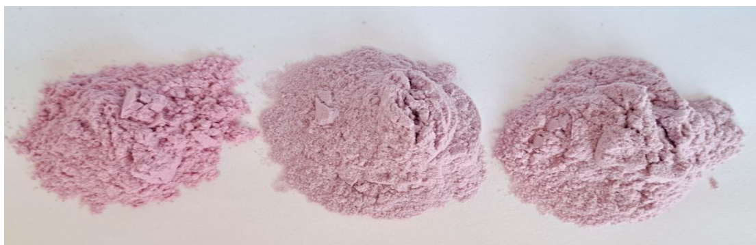
Figure 2. PPCb encapsulated by freeze-drying. a) Using M as wall material; b) Using GA as wall material; c) Using M-GA in a 1:1 ratio (M-GA) as a wall material.
