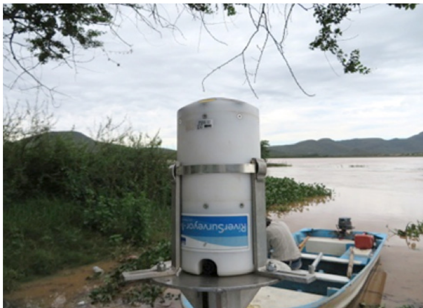
Figure 2. SonTek M9 equipment used to obtain depth data.
