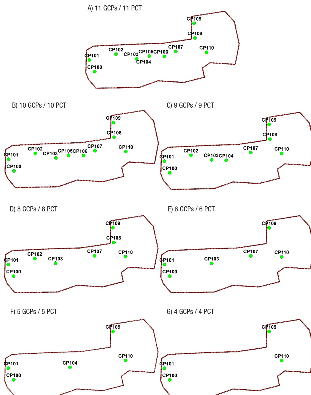
Figure 4. Location of ground control points (GCPs) by the photogrammetric restitution project.
