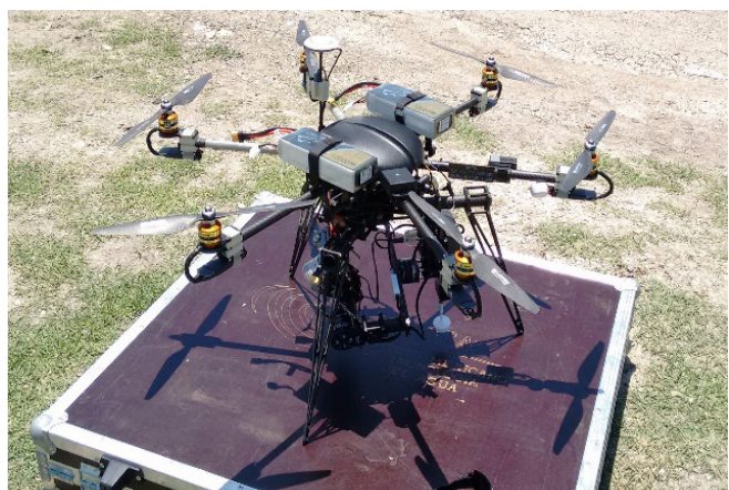
Figure 1. The unmanned aerial vehicle (UAV) Hexacopter and Sony NEX-7 camera.
