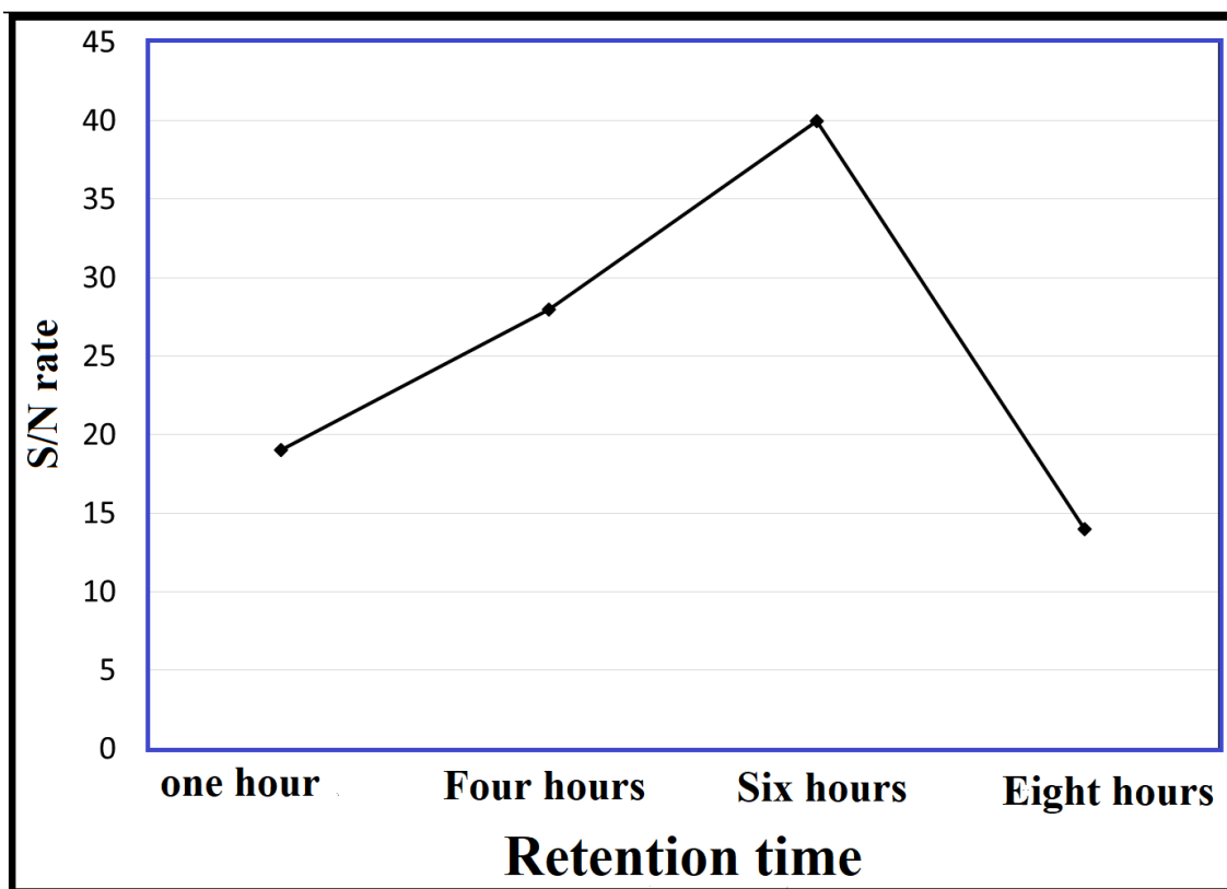
Figure 4: Changes in the efficiency of nitrate removal relative to retention time
