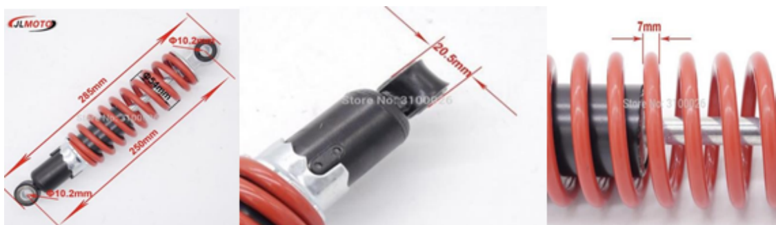
Figure 1: JLMoto brand suspension system dimensioning reference 3100026.
