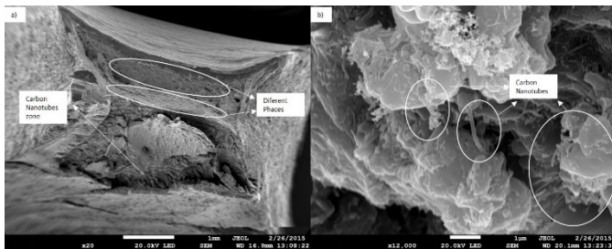
Figure 21: Material processed with circular pin, concave shoulder at 0.5 molar with double deposition layer and 0.5M-O-2C 1P tool pass, a) 20X approach and b) 12000X approach.
