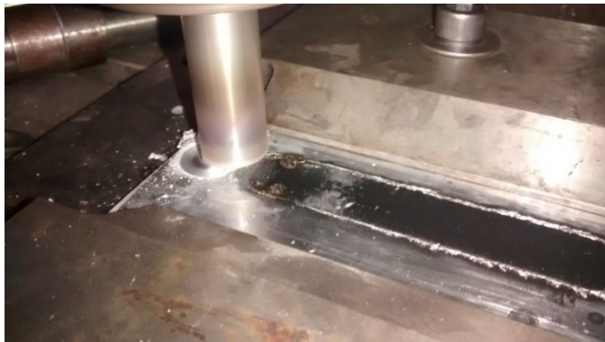
Figure 6: FSP on Aluminum plate with solidified mixture
