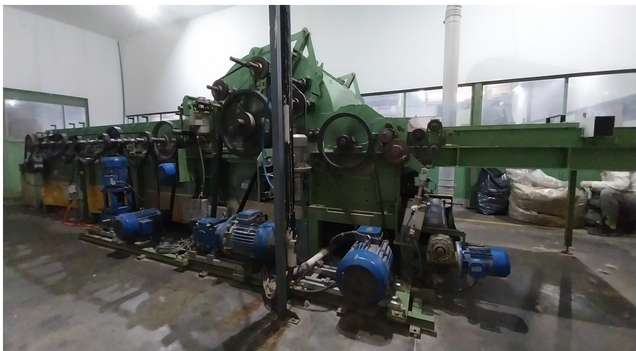
Figure 2. Dehairing machine used for the present study, at a textile company in Argentina.
