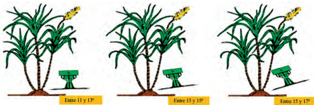
FIGURE 8. Recommended magnitudes of the base-cutter angles (Abadia, 2018).
