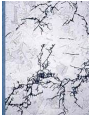
FIGURE 10. Under stress corrosion.
