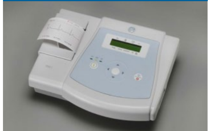
Figura 3. GE MAC i, ECG portable Fuente: http://www3.gehealthcare.in/en/products/categories/diagnostic-ecg/resting/mac-i
