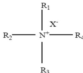
Figure 1.1. General molecular structure of a QAC (R represents a functional group, X<sup>-</sup> represents a counter ion such as Cl<sup>-</sup>, Br<sup>-</sup>, or NO<sub>3</sub><sup>-</sup>)
