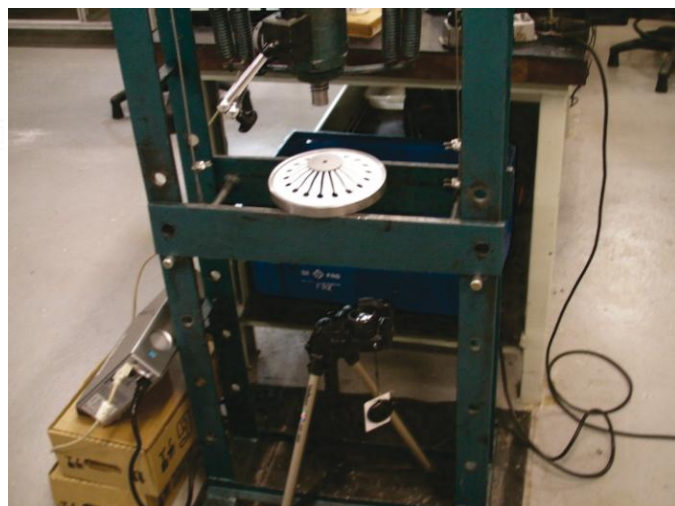
Figure 3 - (a) Experimental setup for shadow moiré tests and (b) equipment positioning
