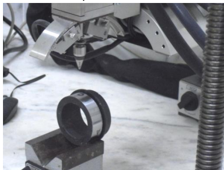
Fig. 2. Analyzer of stresses Stresstech, model X stress 3000
