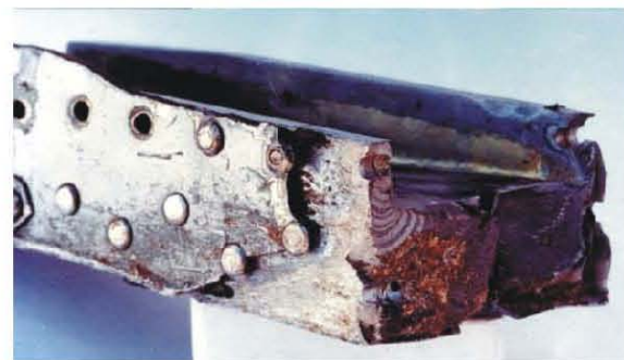
Figure 2: AT-26 wing main spar failure (Mello Jr., 1999).
