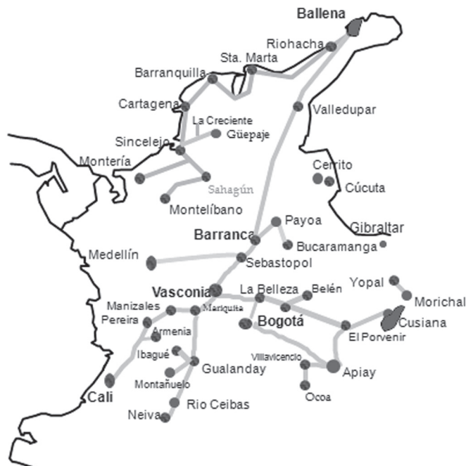
FIGURE 2. COLOMBIAN NATURAL GAS PIPELINE SYSTEM (GUTIERREZ, 2008)
