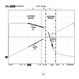
Figure 6. Measurement in the reset period. (a) Applying a saw-tooth voltage signal  $(V_{IN})$  directly to the FG terminal by using the access switch. (b) Graph of the inverter's output transient response
