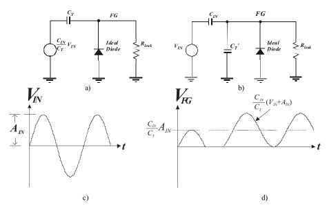
Figure 5. (a) Simplified circuit. (b) Thevenin reduction. (c) Periodical input. (d) V<sub>IN</sub> contribution to the FG potential, V<sub>FG</sub>
