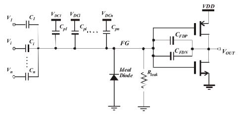
Figure 3. Equivalent circuit for a multiple-input FG-CMOS inverter using a N-channel MOSFET as a real analog switch
