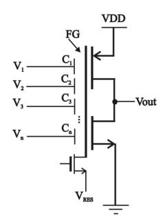
Figure 1. Electrical Diagram of a Clocked-Controlled FG-CMOS Inverter
