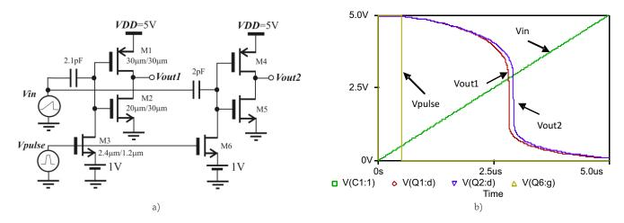
Figure 9. A simulation example, a) Two similar CMOS FG Inverters M1=M4, M2=M5 and M3=M6 with a slight difference at the input capacitance, b) The inverters simulation response using Transient Analysis on PSpice
