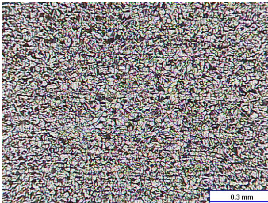
Figure 4. Microstructure of the plain carbon steel at 100X.
