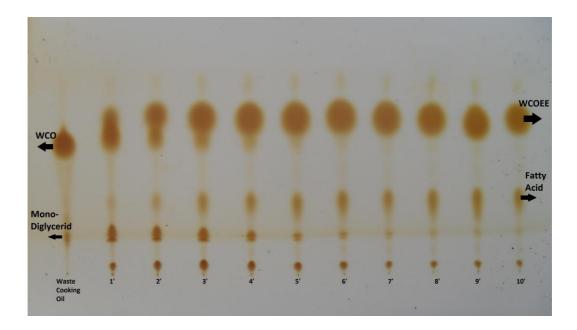
• Figure 1. Thin Layer Chromatography (TLC), using silica gel coated aluminum foils from Merck and a mixture of hexane: ethyl acetate (95:5).
