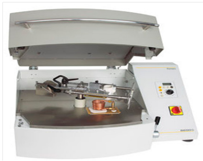
Figure 3 (a) BEGO induction furnace in argon atmosphere. (b) Actual photograph of the furnace arm.
