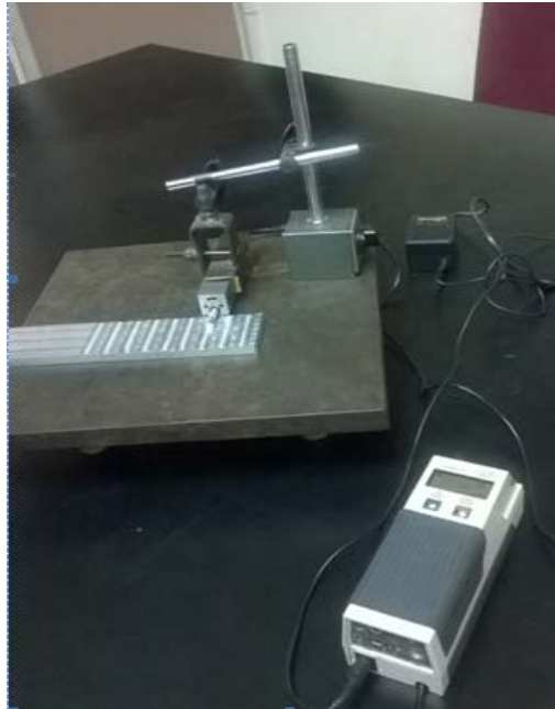
Figure 4: Measurement of surface roughness using Surf Test-211 series (Mitutoyo)
