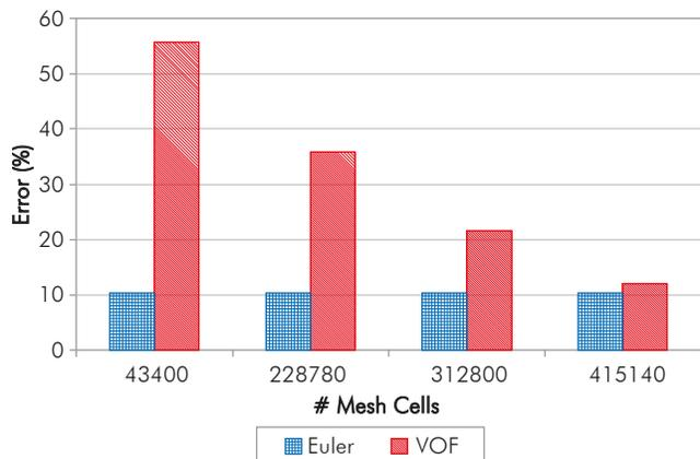
Figure 4. Mesh independence test – Experimental and CFD results comparison
