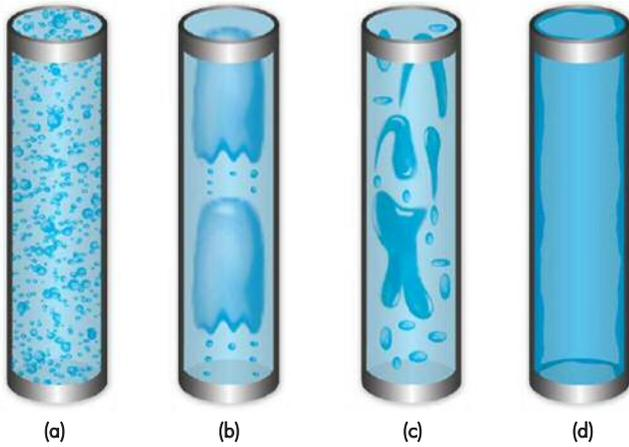
**Figure 1.** Flow patterns in vertical pipes.
