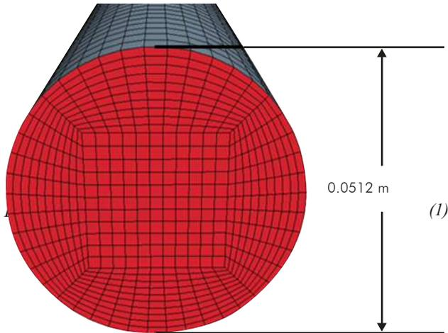
Figure 3. Orthogonal (Butterfly) grid
