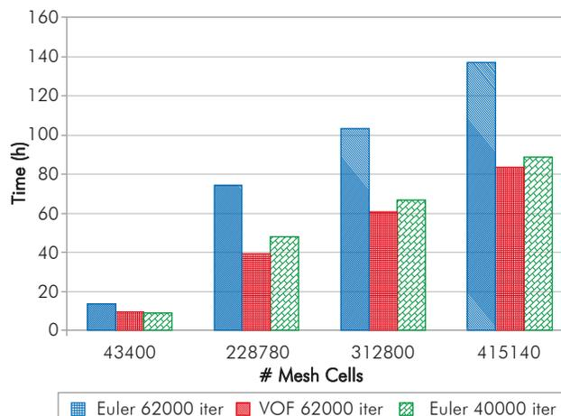
Figure 5. Mesh independence test – Simulation time
