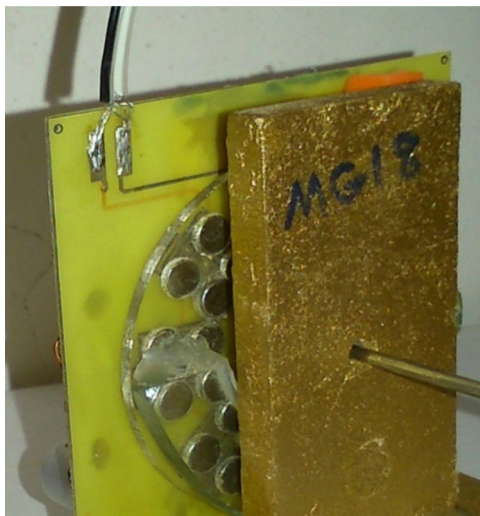
Figure 12. Laboratory model of the proposed microgenerator.
