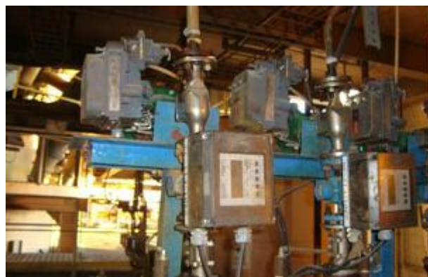
Figure 4: individual flowmeters in each line of the dosing system with centrifugal pumps
