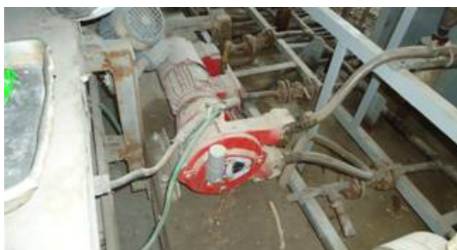
Figure 5: Peristaltic pump SPX10 installed for the tests
