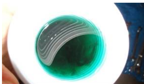
Figure 8: Oil condition after 8 months of operation
