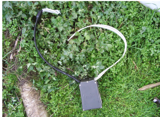
Figure 2. Detail of GPS-GPRS collar.
