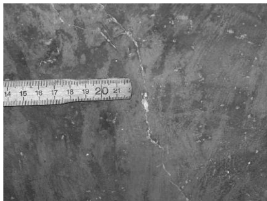
Fig. 2 Irregular and inhomogeneous alteration of azurite into paratacamite.
