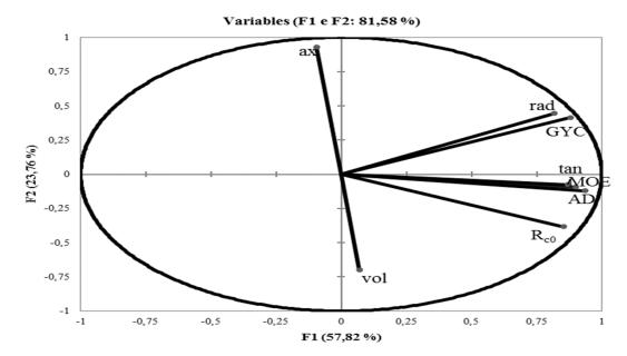
Where:  $R_{c0}$  = resistance to the parallel compression to the charcoal fibers, MOE = module of elasticity. tan = tangential linear degradation, rad = Radial linear degradation, ax = Axial linear degradation, GYC = Gravimetric yield, AD= apparent density
