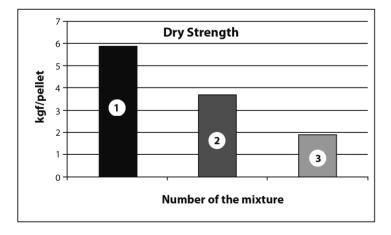
Figure 3 Dry pellets strength as a function of the test number.
