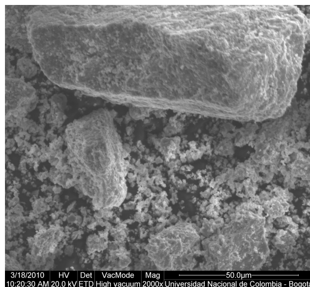
FIGURE 2. SEM micrograph of \text{La}_2\text{SrCo}_2\text{FeO}_9 obtained from ETD detector (secondary electrons).
