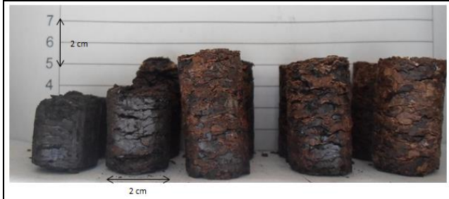
Figure 2. Coal- cocoa pod husks pellets made from intermediate particle size and organized by the cocoa content in the blend (0,30,50,70 and 100% wt from left to right).
