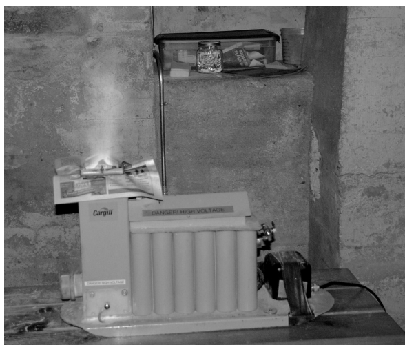
Fig. 4. A flour dust explosion demonstration. The top of the building had been tightly covered with two layers of newspaper. The actual explosion blew the paper away and the flames seen here follow immediately, but last only a fraction of a second. The building is about 40 cm tall.
